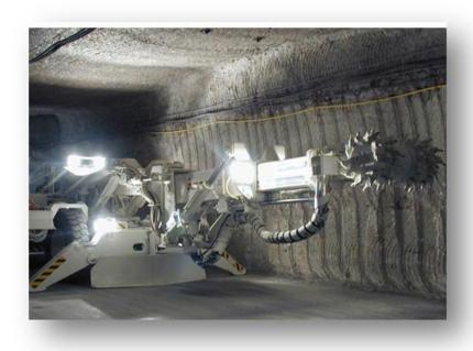
Miners operating seal cutters are well away from the location where the rock is being removed.
